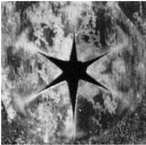
Fig. 12 Beamlet cross section determined by foil erosion method.
